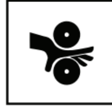
PINCH HAZARD KEEP FINGERS AWAY
